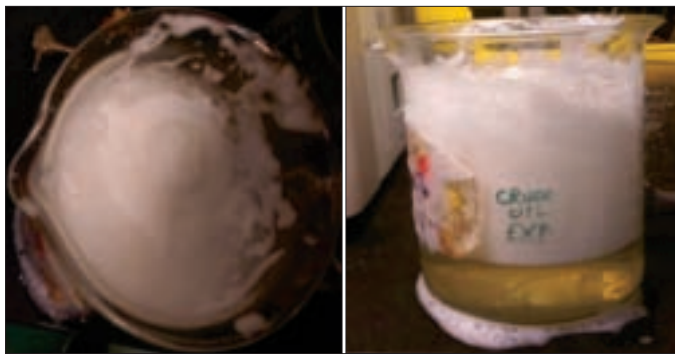
Fig. 4. Collected samples of the foam generated inside the flow loop.
