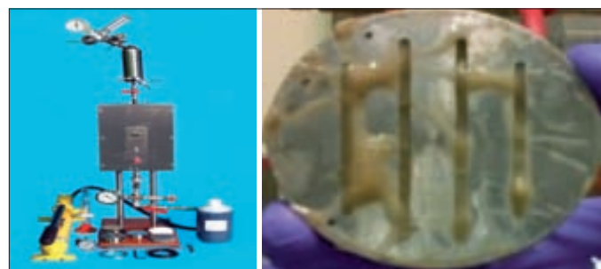
Fig. 3. PPT apparatus and the 2 mm slotted disc used for testing the ARC plug.
